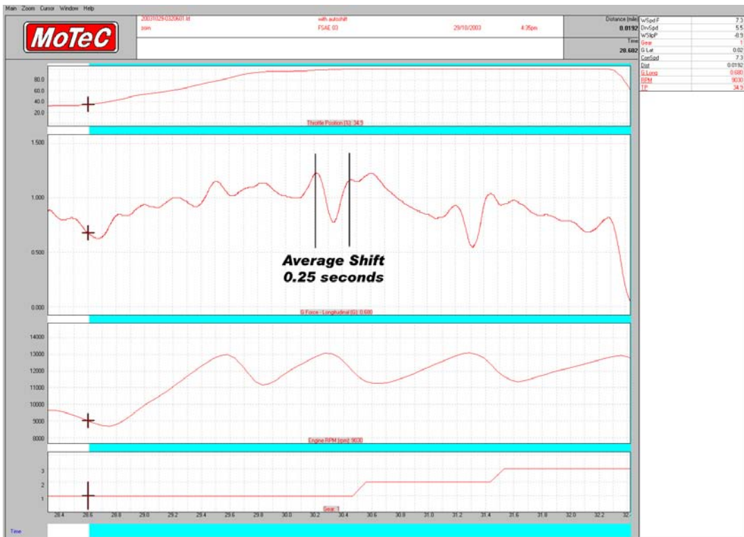
Figure 1: Shift time with automatic upshift feature
